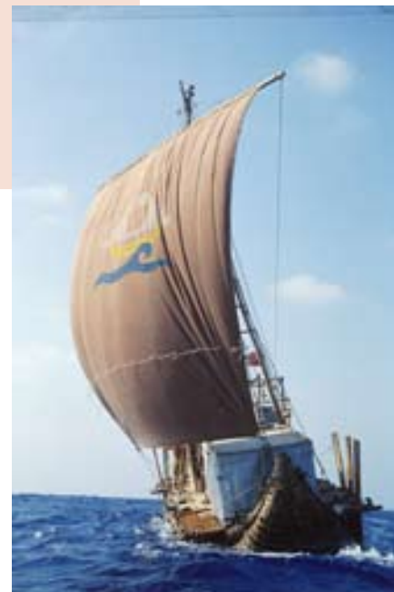
The reed-boat ABORA II tacked against the difficult Mediterranean winds with a 60 m 2 sail area.
